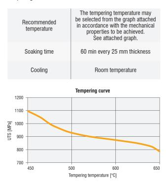
Tempering curve obtained on a test piece austenitised at 890 °C. After tempering it may be useful to carry out a stress relieving cycle at 50 °C less.
