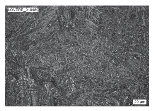
The microstructure of KeyLos® ON detected about 20 mm under surface is tempered martensite.
