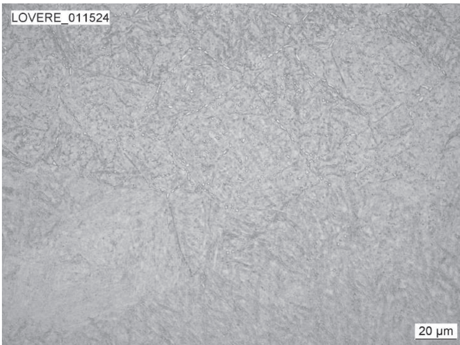
KEYLOS® 2316 in hardening condition: Tempered Martensite with dispersed Carbides
