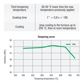
Tempering curve of a sample which has been austenitised at 1040  $^{\circ}$ C. The diagram shows values obtained after the second temper.
