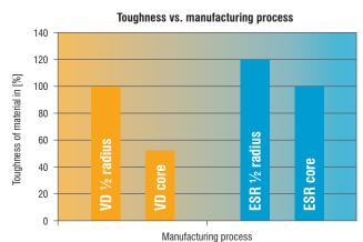
Thanks to the ESR process, EskyLos<sup>®</sup> 2365M satisfies the most difficult requirements in terms of toughness and suitability to polishing. It is suitable for the manufacture of moulds subjected to mirror polishing and to high mechanical stress.
