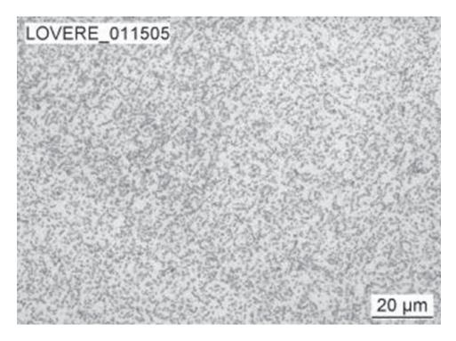
The annealed microstructure of the as received steel consists essentially of a ferritic matrix with a homogeneous distribution of spheroidized carbides, when examined at 500X, after being polished and eetched with 4% Nital, free of excessive banding
