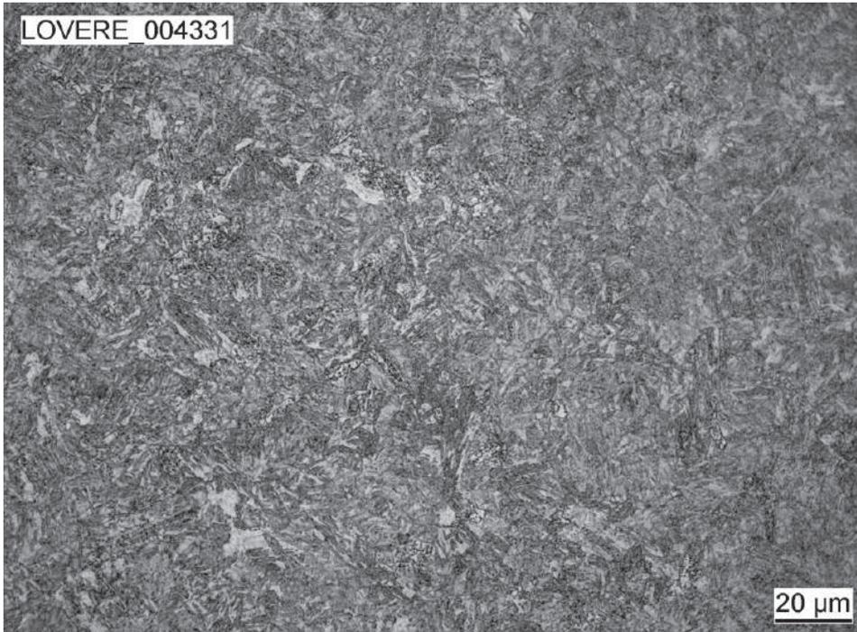
The microstructure of BeyLos® 2711, after hardening, detected about 20 mm under surface is tempered martensite.
