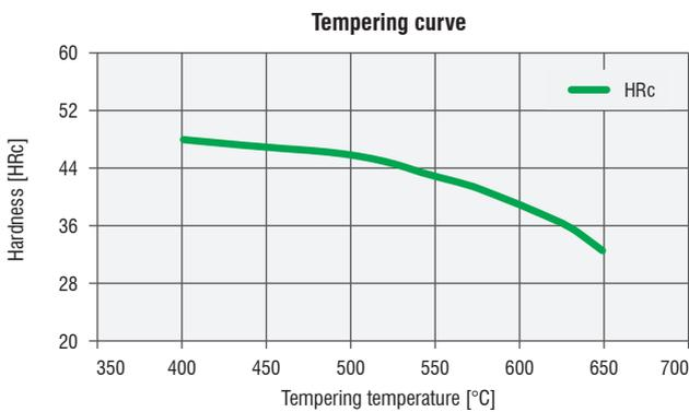
Tempering curve of a sample which has been austenitised at 850 °C and quenched.
