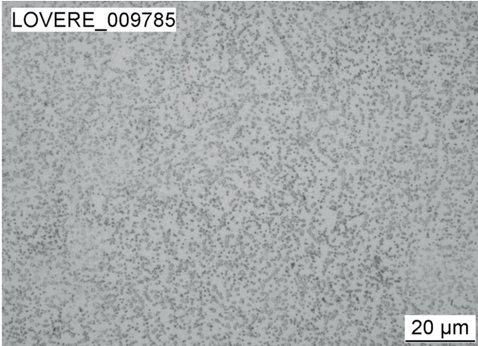
The annealed microstructure of the as received steel consists essentially of a ferritic matrix with a homogeneous distribution of spheroidized carbides, when examined at 500X, after being polished and etched with 4% Nital.
