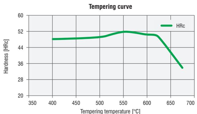
Tempering curve of a sample which has been austenitised at 1040 °C. The diagram shows values obtained after the second temper.
