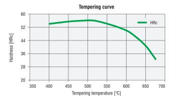
Tempering curve of a sample which has been austenitised at 1020 °C. The diagram shows values obtained after the second temper.
