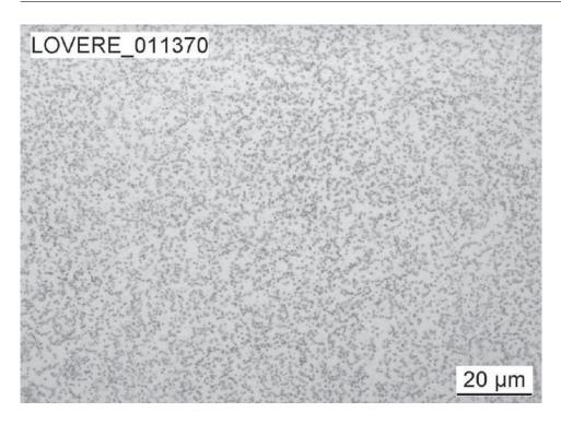
The annealed microstructure of the as received steel consists essentially of a ferritic matrix with a homogeneous distribution of spheroidized carbides, when examined at 500X, after being polished and etched with 4% Nital, free of excessive banding.
